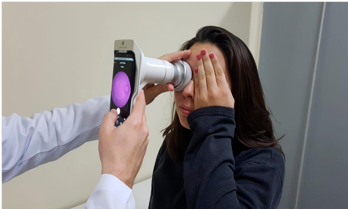
Figure 102: Device positioning for retina image capture
